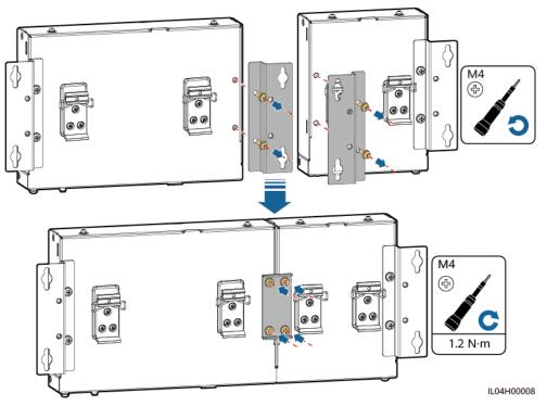
Step 2 Install the SmartLogger and SmartModule.
