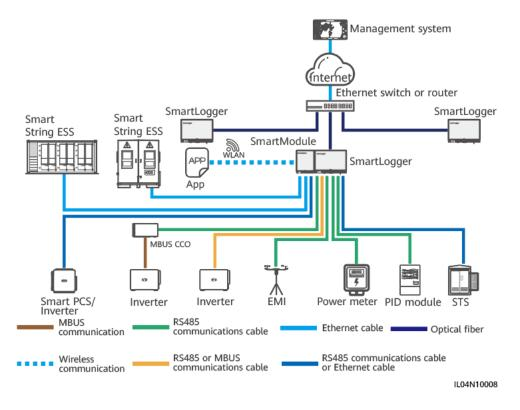
Figure 2-4 Fiber or Ethernet star network
