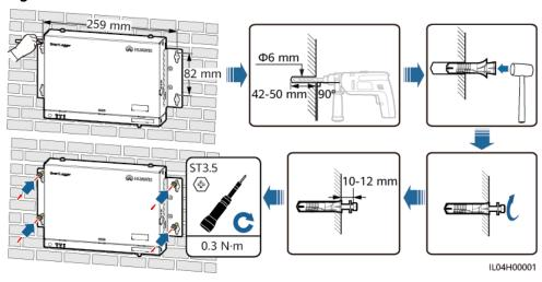
Figure 3-2 Wall-mounted installation
