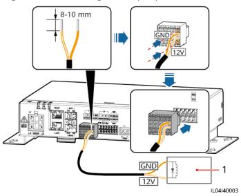
Figure 4-7 Connecting the output power cable
