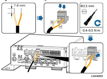
Figure 4-17 Connecting an RS485 communications cable
