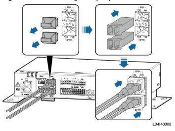
Figure 4-11 Connecting fiber jumpers
