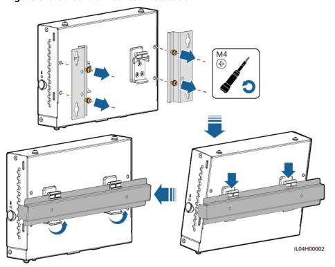
Figure 3-3 Guide rail-mounted installation
