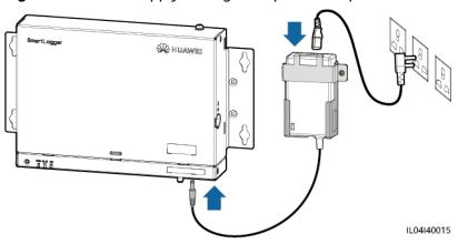
Figure 5-1 Power supply through the power adapter
