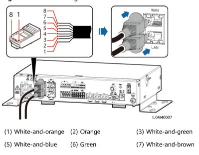
Figure 4-10 Connecting an Ethernet cable
