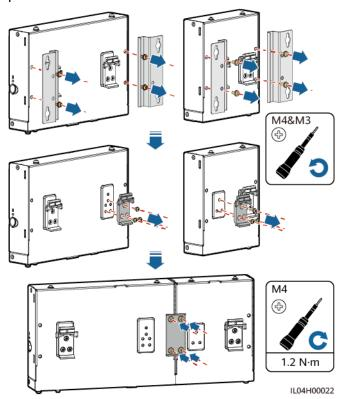
**Step 2** Install the SmartLogger and SmartModule.
