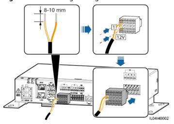
Figure 4-6 Connecting a DI signal cable
