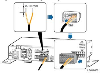
Figure 4-9 Connecting a DO Signal Cable
