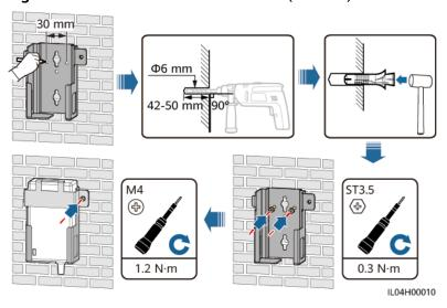
Figure 3-10 Wall-mounted Installation (Mode 2)
