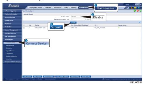
Figure 6-45 Setting parameters for a built-in MBUS module
