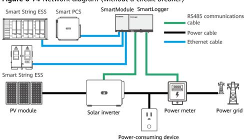
Figure 6-74 Network diagram (without a circuit breaker)
