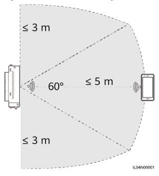
Figure 8-1 WLAN connection range
